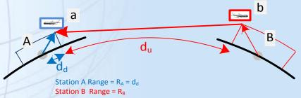
✓ Minimum separation between stations A and B: Range A + Radio horizon A + Radio Horizon B +Range B
